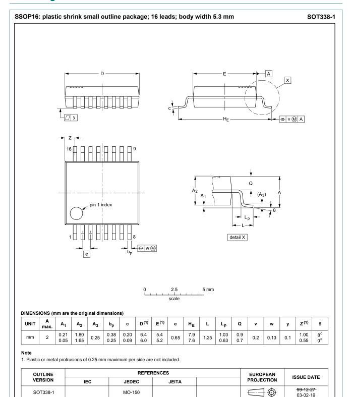
Fig. 1. Package outline SSOP16 (SOT338-1)
